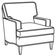
CD88 Series / CD8805T Chair (32W) Outside: 32W x 39D x 37H Inside: 21.5W x 22D
